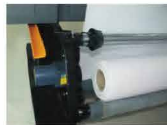
Three feeding methods can be selected according to needs: Insert type, two-roller deposit type, three-roller dragging deposit type
